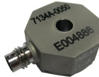
The **Model 7134A** is a true case isolated triaxial IEPE accelerometer available in ±50g to ±500g dynamic ranges. The accelerometer features three internally shielded accelerometer assemblies for superior noise isolation. The assemblies are installed in a hermetically sealed light weight Titanium housing with a 4-pin Microtech connector interface. The model 7134A features piezo-ceramic crystals in annular shear mode which provide a flat frequency response up to >7kHz.
